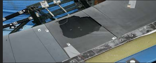
Damage from a simulation of the foam hitting the wing at 525 mph.
