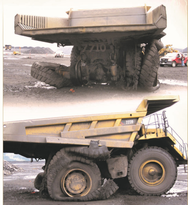
27.00R49 tires after a lightning strike. The four rear tires blew out immediately. The left rear out tire was propelled 820 ft and the wheel 985 ft. The “hidden danger” is in the front tires.
